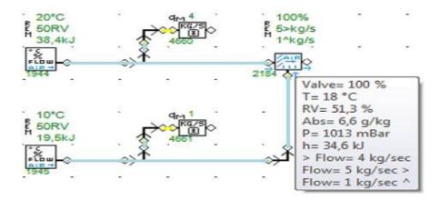
Examples source 1944 for flow (4 kg / sec) 20'C is mixed with 1945 source flow (1 kg / sec) 10'C Setting Parameter Mixer% = 100%.
