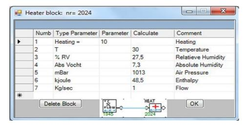
Block Parameter Heating Heat which you can set how many degrees the air must be heated the air must be heated be.
