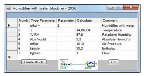
Block Humidifier allows you to Parameter g/kg = can set how many grams of water per kg air humidified air should be come. In this example you can see that the temperature drops from 25 degrees to 19.8 "C by extracting vapour heat absolute humidity increases from 7.3 to 9.3 and from 36.9% RH to 64.3. Enthalpy of the air remains the same.
