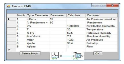
Fan unit with which you can set with Parameter = mBar how the pressure is increased In this example you can see that the air pressure is increased from 1013 to 1023 mBar. Everything under Calculate automatically calculated. Through change air pressure also changes %R.V a little. Look under calculate kw automatic calculate Power needed for the Fan: 1.38 kW. The block has one input and one output.
