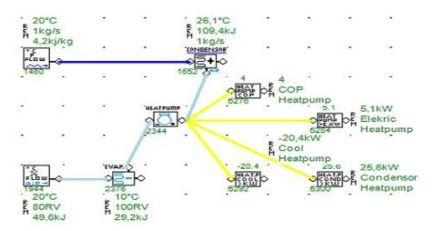
Applying Heatpump Air > Water
